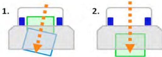
Independent pick rollers ensure a skewed document will not affect the alignment of following sheets
