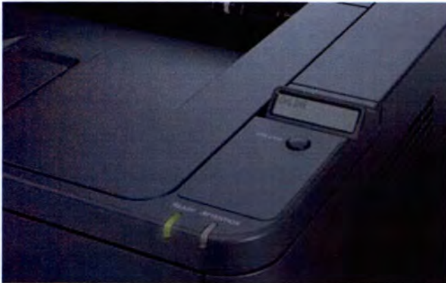
B411d/dn operator panel: 16-character x 2-line LCD display; access to printer status and functionality via printer driver on PC
